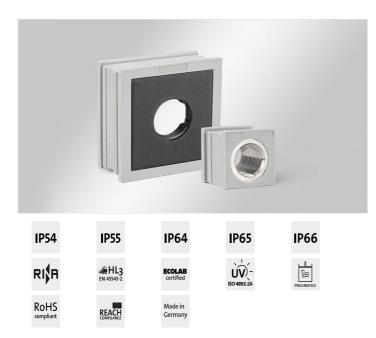
AT-M is an adapter grommet (based on large KT grommets) with integrated metric threads.. The AT-M adapter grommets are made of elastomer with a polyamide body. AT-M adapter grommets are available with inner threads M12 x 1.0, M16 x 1.5, M20 x 1.5 and M25 x 1.5.
